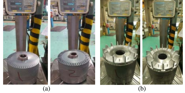
Fig. 4 Weight measurements of (a) rotor core, dummy shaft, and (b) rotor assembly for die cast rotor FF estimation
